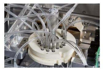
High-quality shear-valve ensures accurate blood volume collection for highest precision on results.
