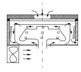
Proprietary design of dual path ventilation enforcing air cooling from both the upper and lower side for the rotor.
