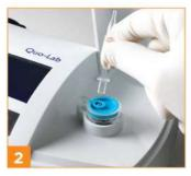
When prompted press reagent bead into cartridge using the reverse end of the sampling tool.
