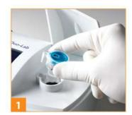
Scan lot calibration barcode. Remove foil from cartridge and insert into analyzer.
