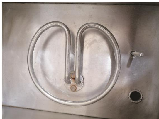
Heater & Level sensor
